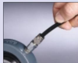
5. And plug the tube into the Quicklinc™ adapter
