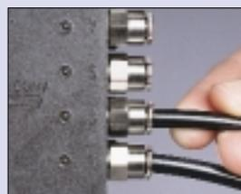
1. Install a Quicklinc™ into the diverter valve and insert the line
